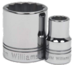
1/2 Drive Shallow Socket, High Polished Chrome Finish, 12 Point, 15 mm JHWSTM-1215
